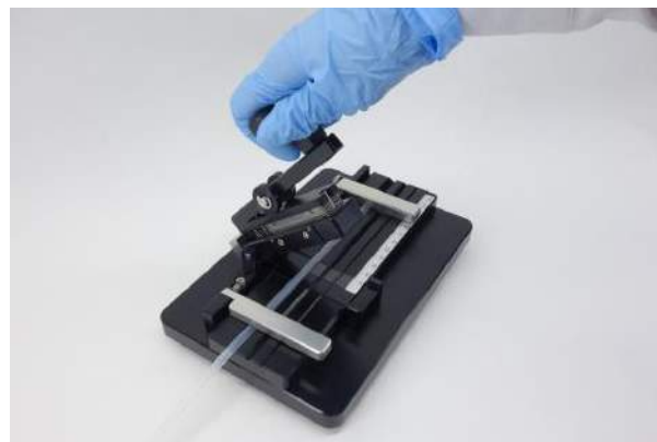
▲ Showing how to cut a silicone catheter
